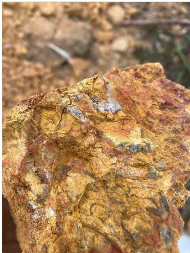
Photo 10: Extremely weathered sandstone recovered from test pit TP06.
