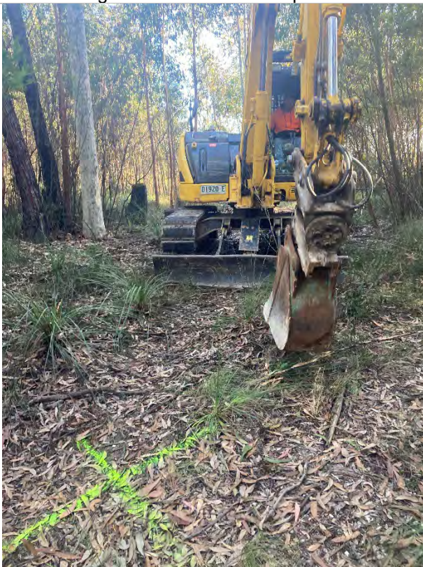
Photo 7: Sumitomo 8-tonne excavator used for test pit excavation in the Phase 2 development area.
