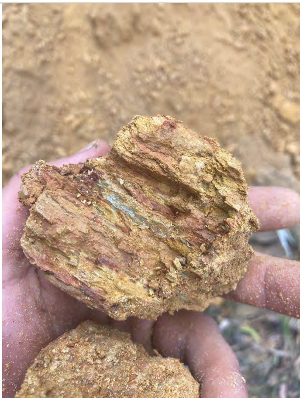
Photo 9: Extremely weathered siltstone recovered from test pit TP02.
